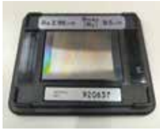
Roughness Specimen 3 \mu\text{m}
